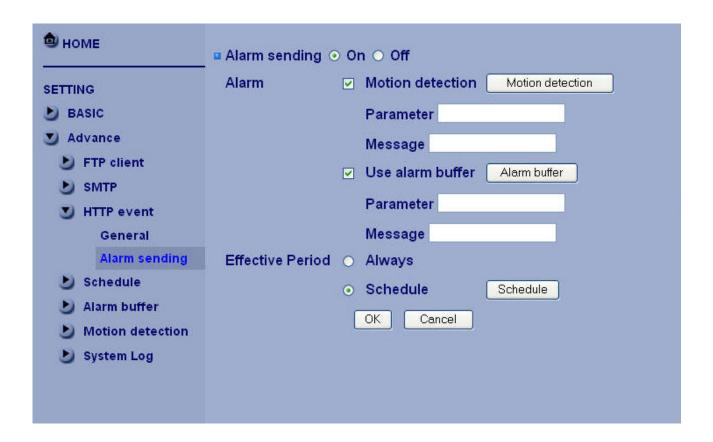
Alarm sending: Select On to set to send mail with connection to the alarm detection.
